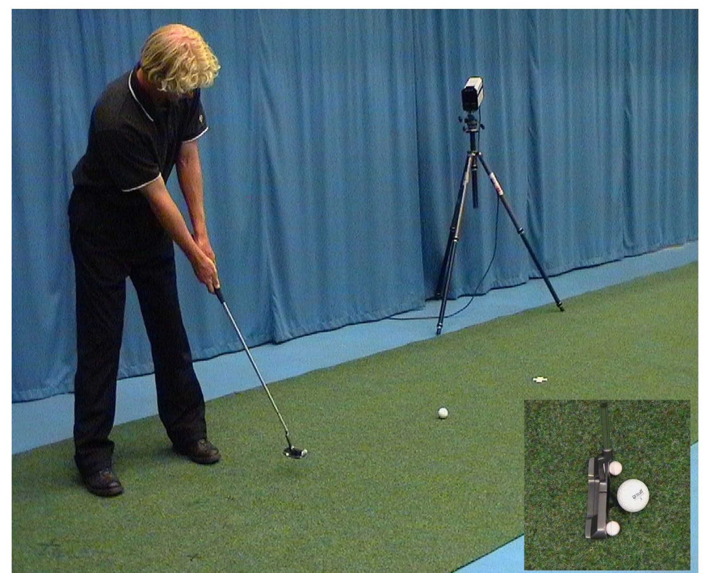
Figure 2: Putting test setup. Inset figure; top view of putter head with reflective markers.
